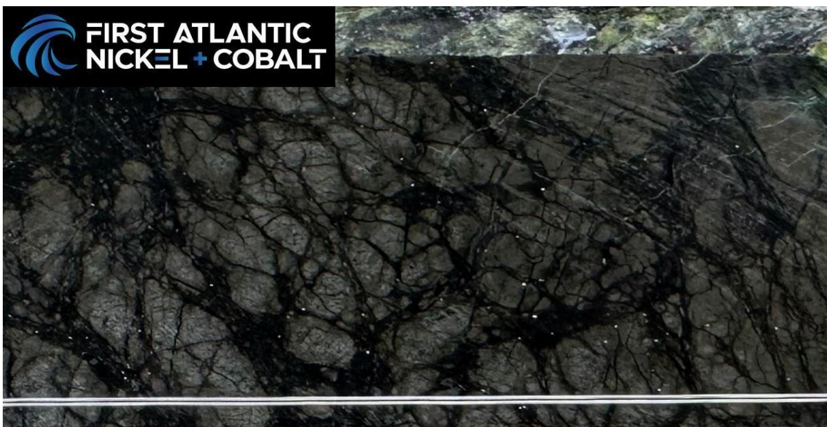
Figure 2: Drill core from the Pipestone XL Nickel-Cobalt Alloy Project showing visible coarse-grained awaruite (Ni-Fe-Co alloy)
